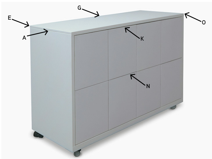
Figure 1. The cabinet used in the tests shown with arrows indicating the points for the push and pull actions.
