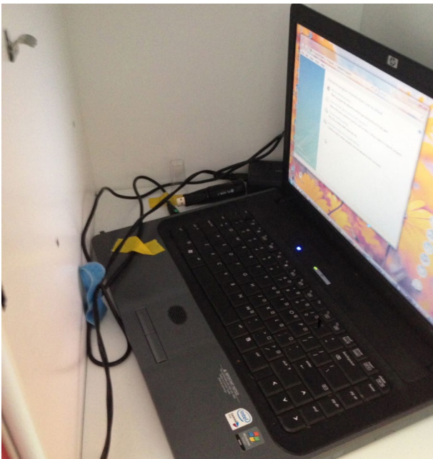
Figure 5: HP 530 Notebook PC setup inside locker with the temperature logger placed close to the laptop, near the exhaust vent of the laptop's cooling fan. Items of clothing and paper were placed inside all adjoining lockers (results shown in Fig 4).
