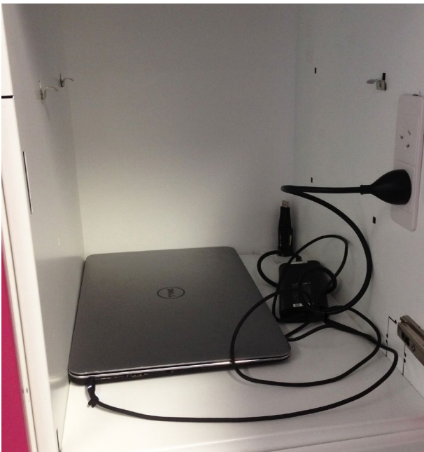
Figure 3. Dell Precision M3800 laptop setup inside locker with temperature logger in the right hand corner (results shown in Fig 1).
